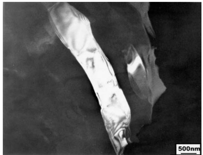
Fig. 8 Dark field TEM micrograph of the columnar grain morphology exhibited by \alpha - \text{Al}_2\text{O}_3
